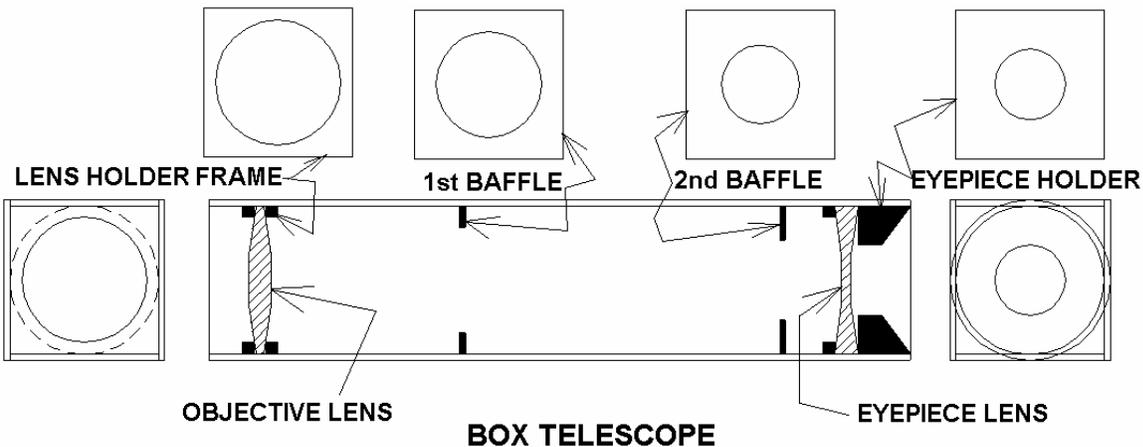
Paint the insides of the tube flat black. The baffles are used to keep stray light from glaring up the insides of the tube, which then reflect into the eyepiece. These baffles effectively trap the unwanted light. Generally speaking, the more baffles, the better the image contrast.
